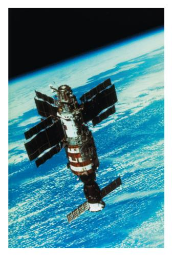
The Salyut 7 space station photographed in orbit. Attached to the space station at the bottom, with the separate solar panels, is the Soyuz T14 ferry spacecraft. Soyuz T14 was launched on September 17, 1985 and carried cosmonauts Vladimir Vasyutin, Alexander Volkov, and Georgi Grechko to Salyut 7. Their mission was terminated when Vasytin became seriously ill, and they returned to Earth on November 22, 1985. Photo Researchers, Inc. Reproduced by permission.
